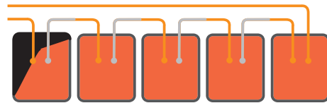
SERIES CONNECTION. All of the modules perform as the worst performing module of the group: there are losses due to mismatch and partial shading.
